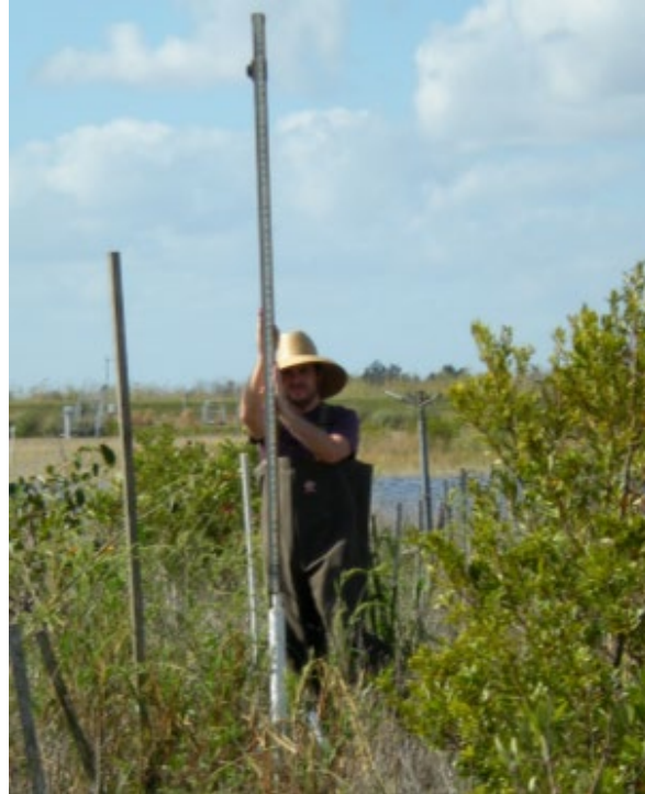
Surveyed the groundwater wells to compare groundwater and surface Water levels
