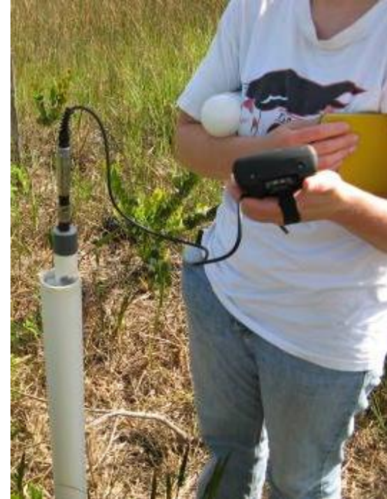
In-situ troll 500 Pressure Transducers were used to monitor water levels
